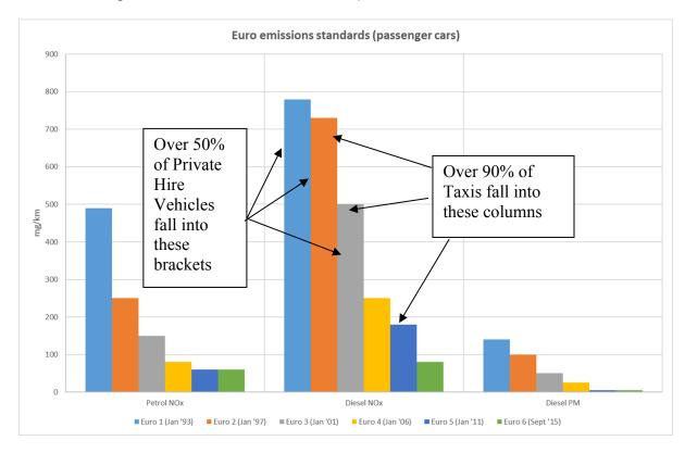
Note: The above graph shows the emissions by Euro Standard and the dates they came in and does not necessarily give the actual emissions in the "real world".
